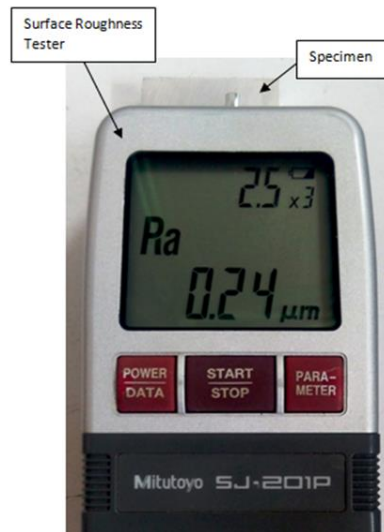
Figure 4: Surface roughness tester
